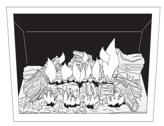
Figure 26. Proper flame pattern.
